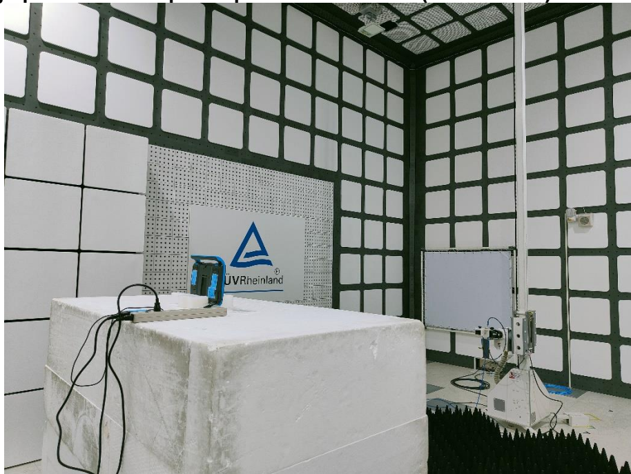
Photograph 6: Test Setup for Spurious Emissions (Back View 4)
