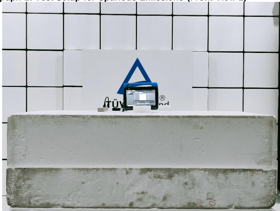
Photograph 2: Test Setup for Spurious Emissions (Front View 2)
