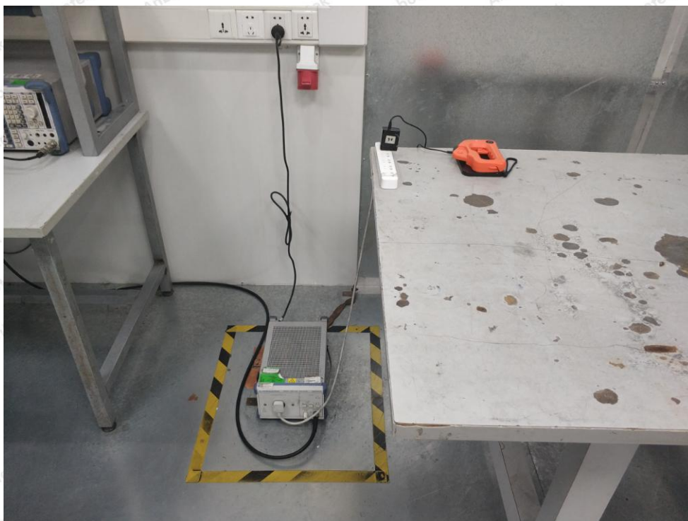
Photo of Radiation Emission Test
