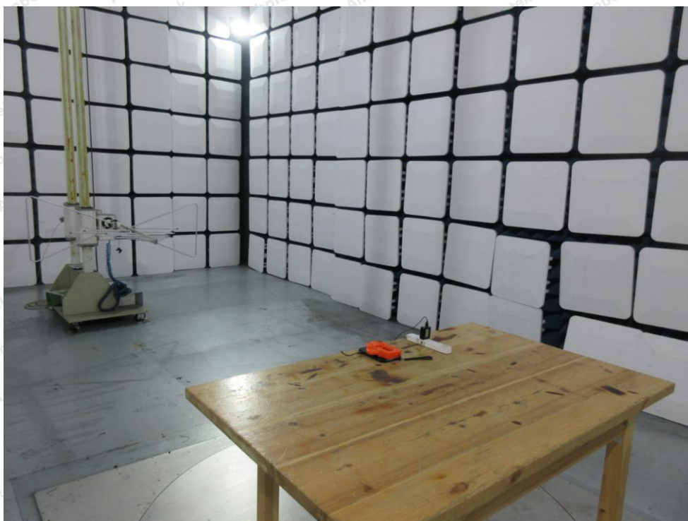
Photo of Radiation Emission Test
