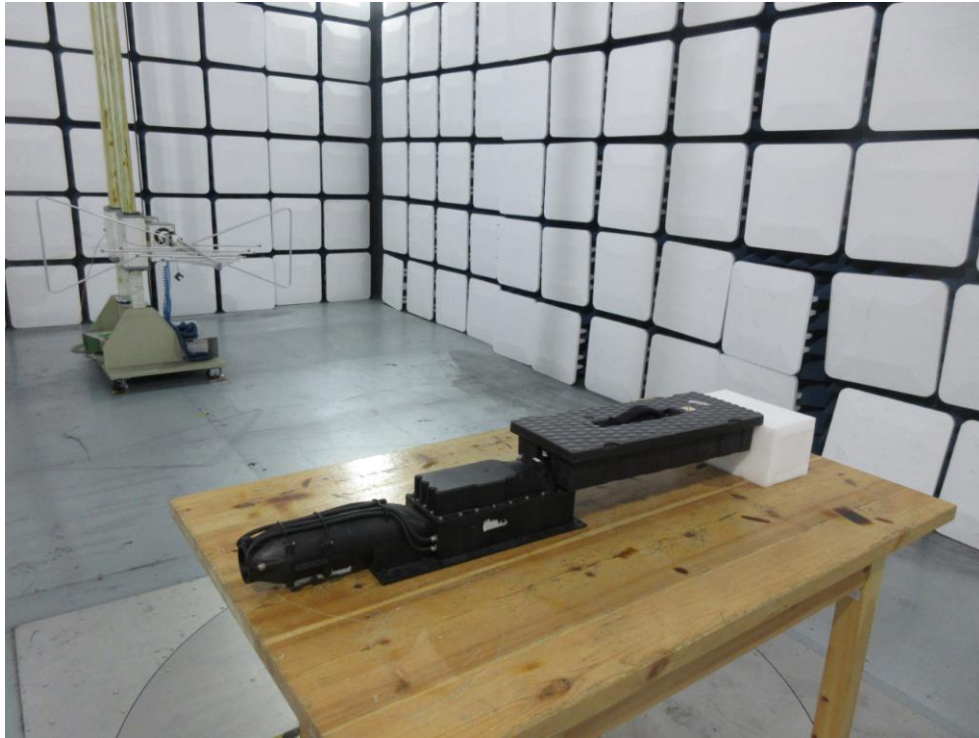
FCC ID: 2AWKQ-YJSDMO1 Photo of Radiation Emission Test
