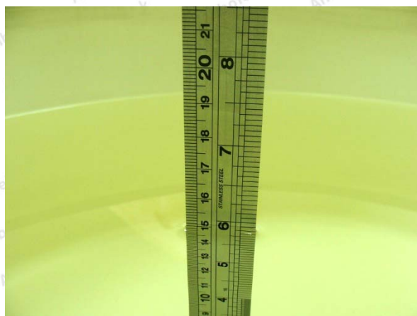
Photo of Liquid Height for Body SAR
