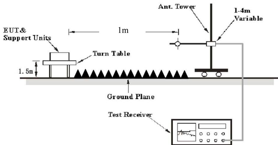
The radiated emission tests were performed in the 3 meters test site, using the setup accordance with the ANSI C63.10-2013. The specification used was the FCC 15.209, and FCC 15.517 limits.
