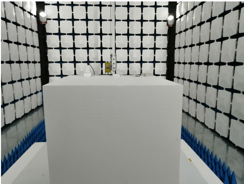
Above 1GHz for radiated emission test setup
