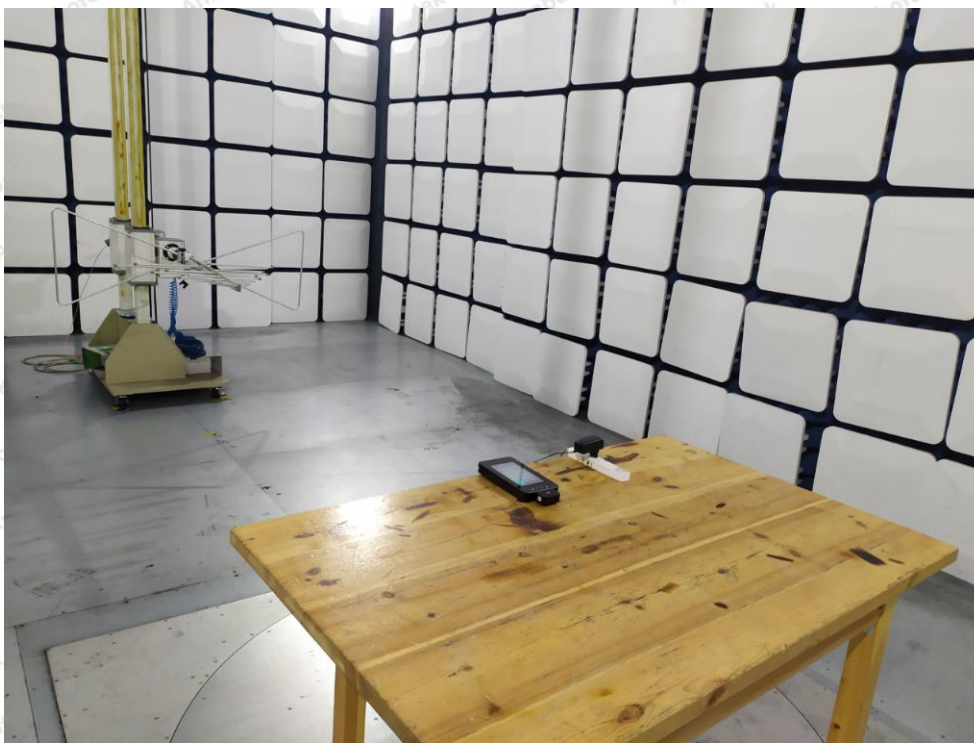
Photo of Radiation Emission Test
