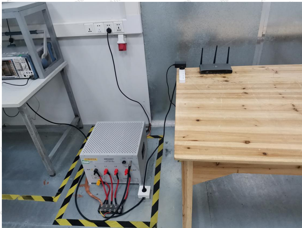
Photo of Power Line Conducted Emission Test
