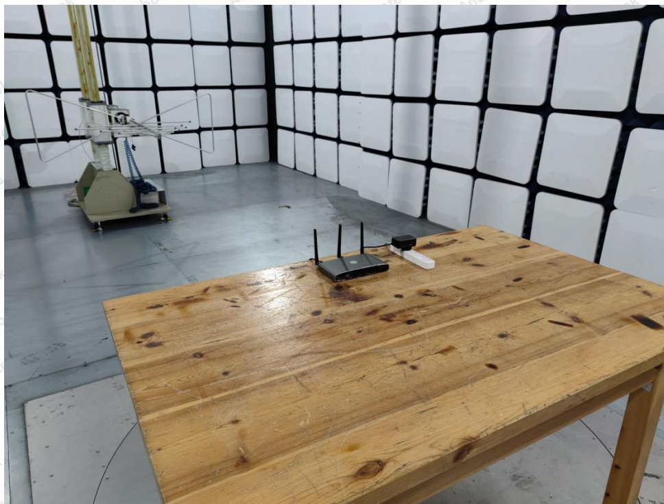
Photo of Radiation Emission Test
