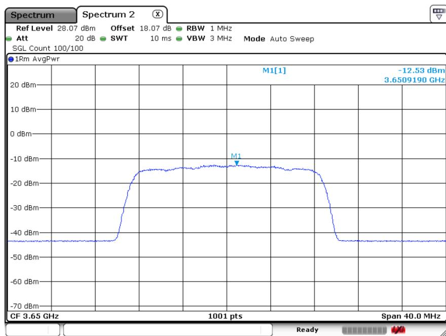
**SAS Granted MaxEIRP 10 [dBm/MHz]****UUT Center Frequency 3650 MHz, Bandwidth 20 MHz, MaxEIRP 9.12 [dBm/MHz]**
