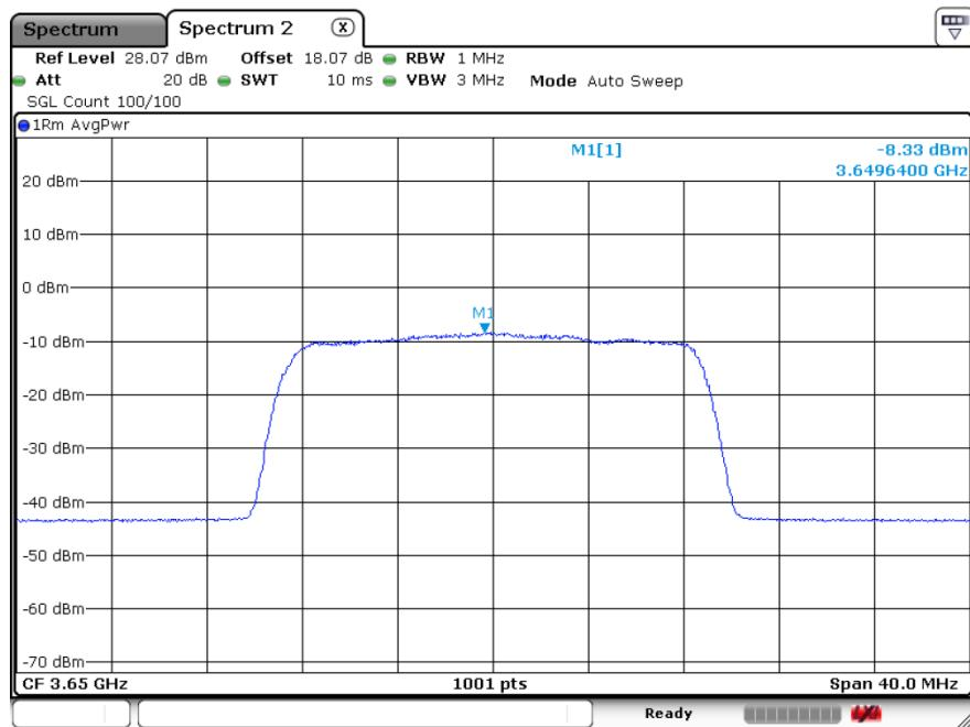
**SAS Granted MaxEIRP 14 [dBm/MHz]****UUT Center Frequency 3650 MHz, Bandwidth 20 MHz, MaxEIRP 11.71 [dBm/MHz]**
