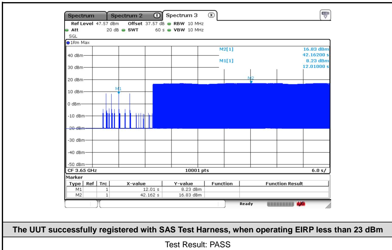
**Note:** The Ref Offset 37.57 dB includes the antenna gain 19.42 dBi and cable path loss 18.15 dB.
