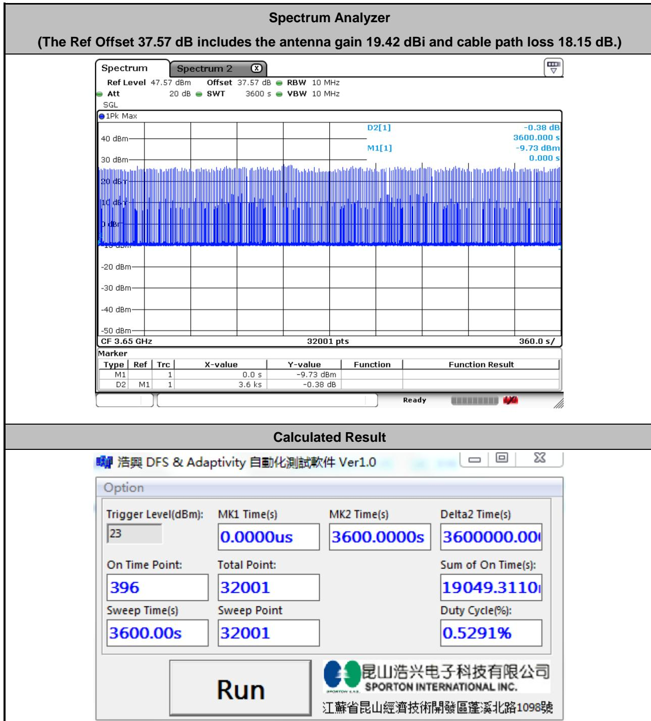
The sum of On Time (aggregated time from marker 1 to 2): 19049.3110ms < 20s, Pass.
