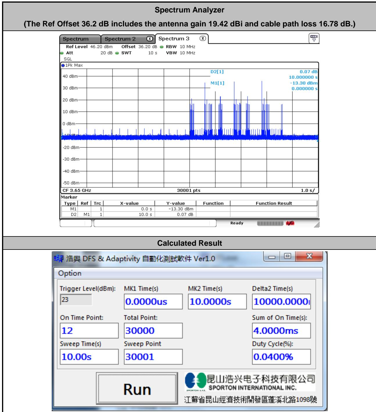
The sum of On Time (aggregated time from marker 1 to 2): 4.0000ms < 1s, Pass.
