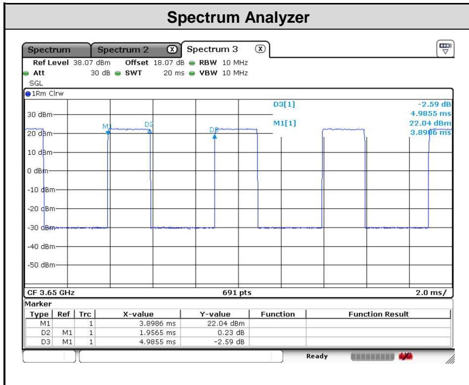
Note: The duty cycle value is 39.24%, add  $10\log(1/\text{duty cycle})$  to the measured power level to compute the average power during continuous transmission.
