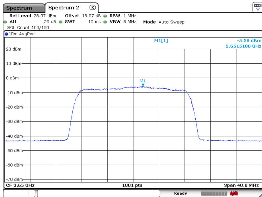
**SAS Granted MaxEIRP 18 [dBm/MHz]****UUT Center Frequency 3650 MHz, Bandwidth 20 MHz, MaxEIRP 16.75 [dBm/MHz]**
