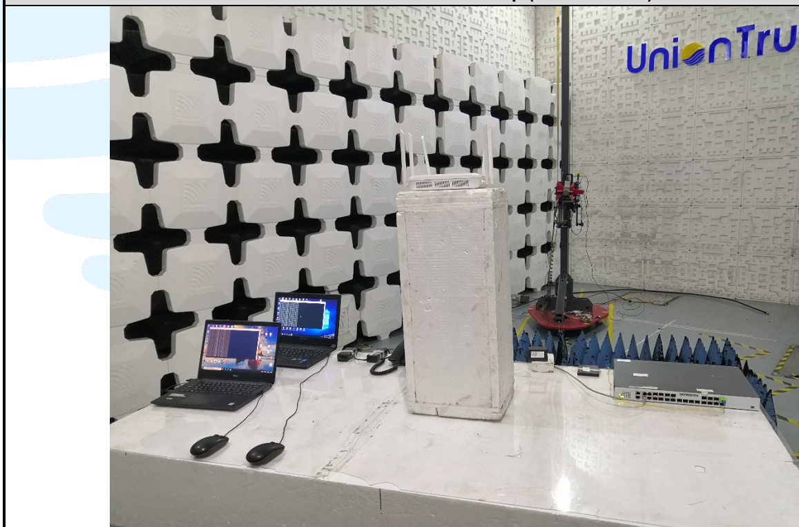
Radiated emission Test Setup (Above 1 GHz)
