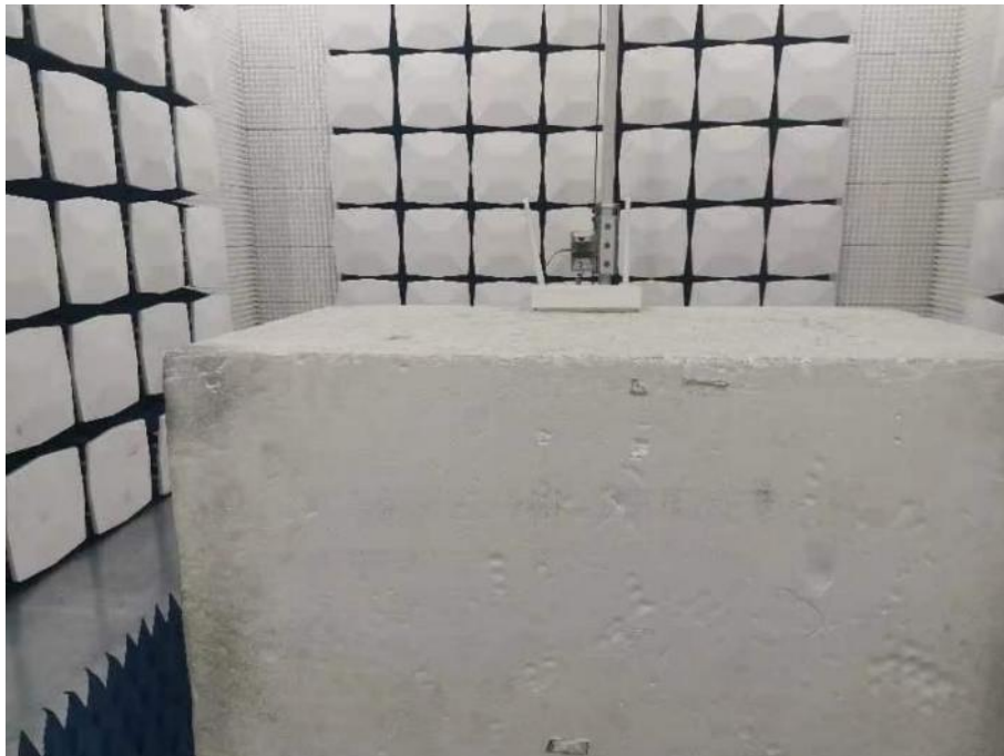
RADIATED EMISSION MEASUREMENT ( Above 1G )
