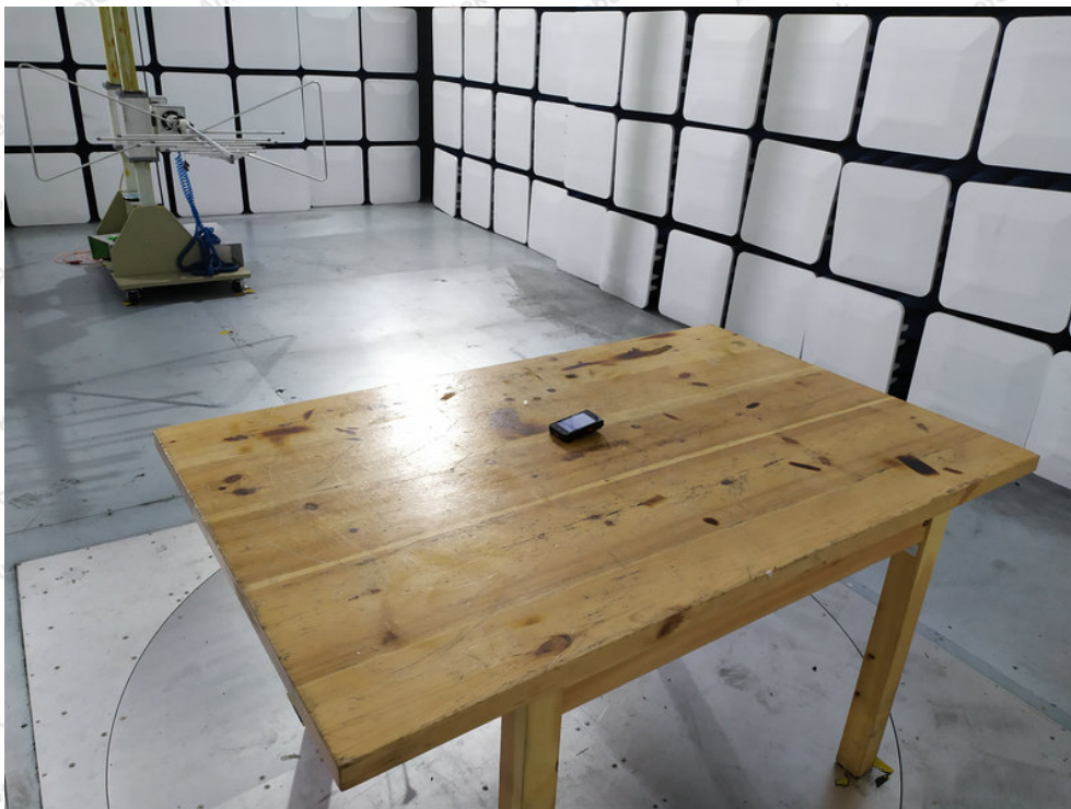
Photo of Radiation Emission Test
