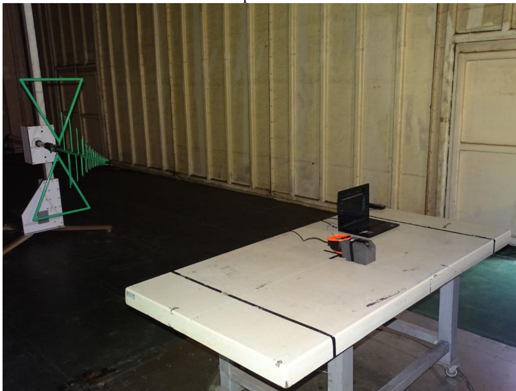
Front View of Spurious Emission Test
