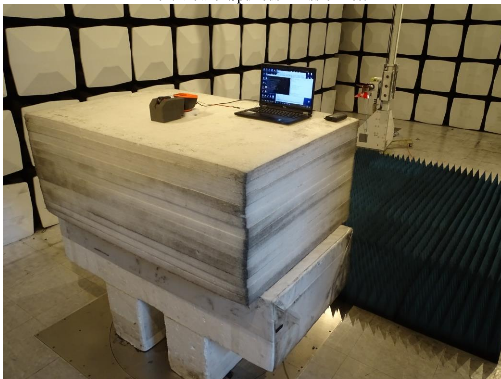
Front View of Spurious Emission Test
