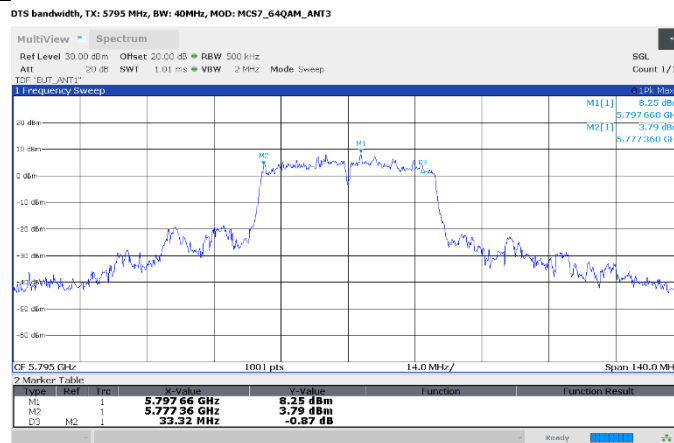
Figure 8.4-3: 6 dB bandwidth, IEEE 802.11n/ac (V)HT40 (CDD) mode, minimum measured DTS bandwidth
