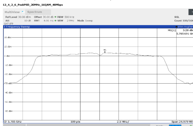
Figure 8.7-5: Power spectral density, IEEE 802.11a (CDD) mode, maximum measured power spectral density
