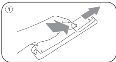
Gently press and hold the circle on the battery cover and push outward to open the battery cover at the back of the remote control
