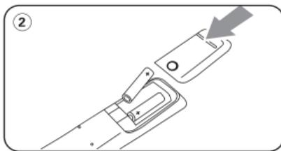
As shown in the figure, put 2 AAA batteries and cover the battery cover (note that the positive and negative battery corresponds to the correct)
