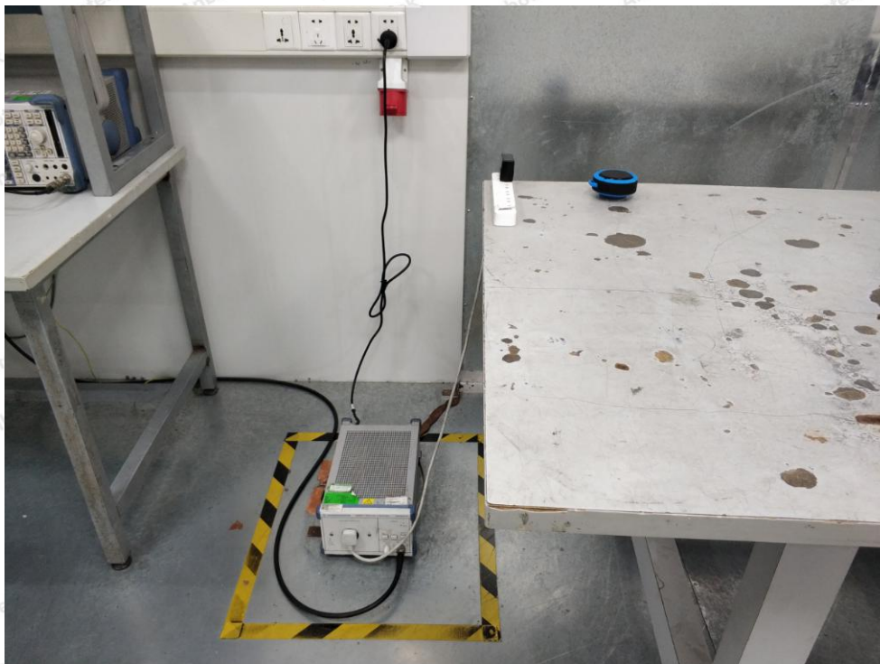
Photo of Conducted Emission Measurement
