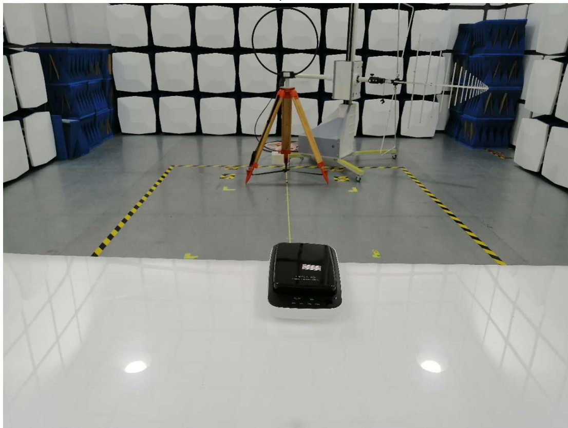
9KHz-30MHz for radiated emission test setup
