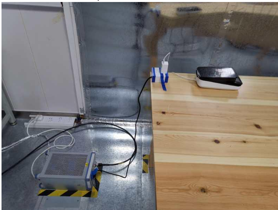
Conducted emission test setup
