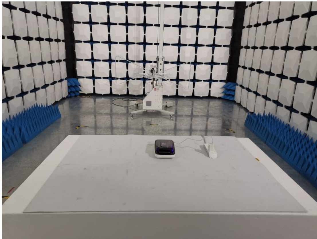
30MHZ-1GHz for radiated emission test setup
