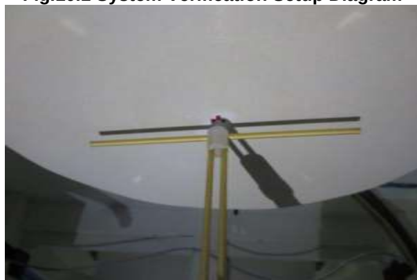
Fig.10.2 Photo of Dipole setup
