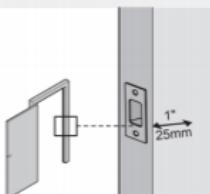
**STEP****2 Install the latch and strike****A Determine backset and adjust the latch**
