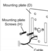
Note: Please support exterior assembly during mounting plate installation.
