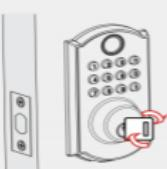
If the keypad and mounting plate are deflected, loose mounting plate screws and adjust.
