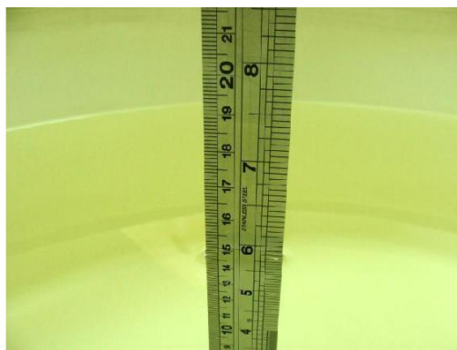
Fig 7.2 Photo of Liquid Height for Body SAR
