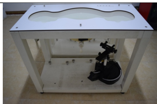
Fig. 6.8 Photo of SAM Phantom
