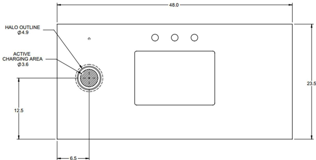
This will guarantee that the end user cannot in normal usage be with 10.7 inches of the charging coils.
