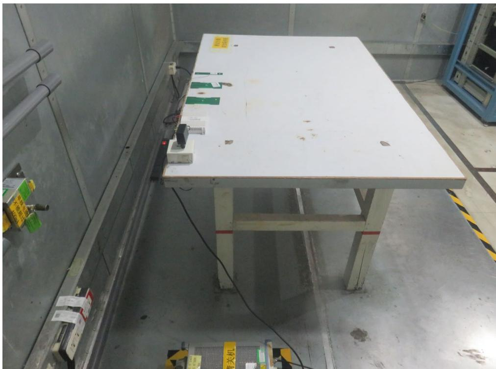
**Radiated Emissions Test Photos****9 kHz to 30 MHz**
