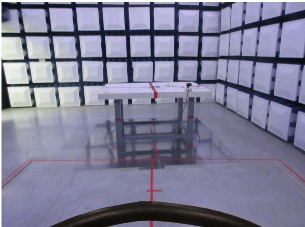
**Radiated Emissions Test Photos****30 MHz to 1000 MHz**
