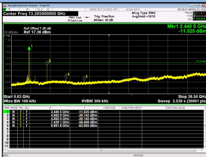
GFSK / High Channel / 30MHz~26.5GHz
