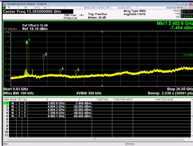
GFSK / Mid Channel / 30MHz~26.5GHz
