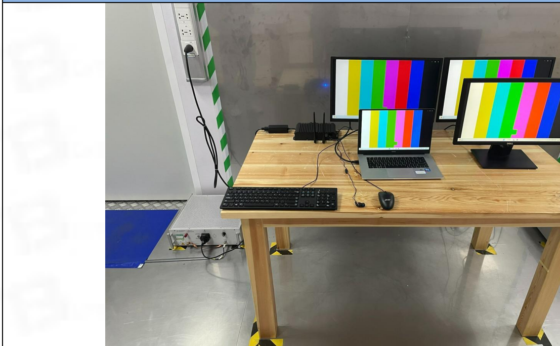
Conducted Emission at AC power line
