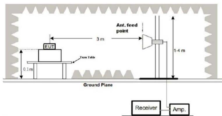
1. For the radiated emission test below 1GHz:
