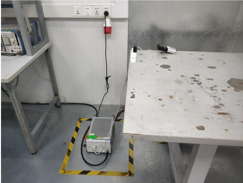
Photo of Power Line Conducted Emission Test
