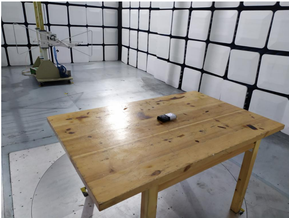
Photo of Radiation Emission Test
