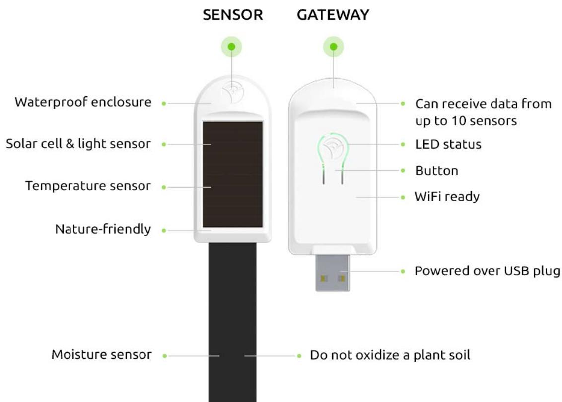
For data transfer plant sensors use gateway, which has WiFi connection and transfer data to the cloud. Gateway can manage data from **up to 10 sensors**. To
