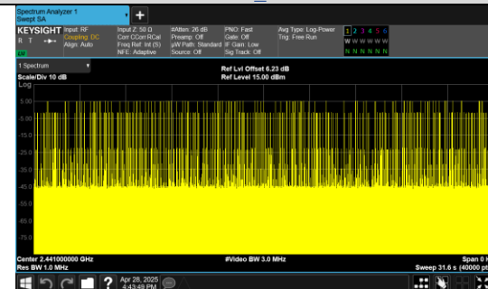
Number of Pulses in 31.6 seconds 8DPSK_3-DH5
