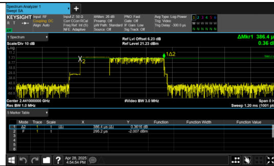
Pulse Width \pi/4 DQPSK 2-DH1
