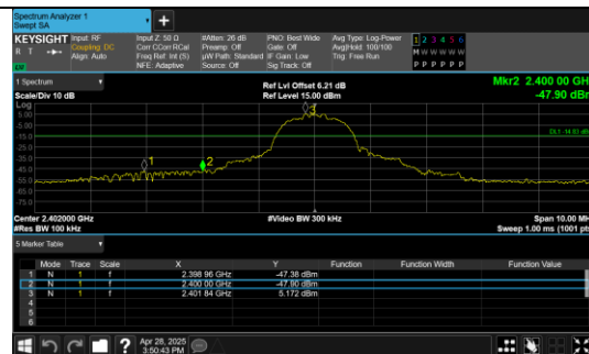
Out Of Band Emission 8DPSK_3-DH5_Channel 0
