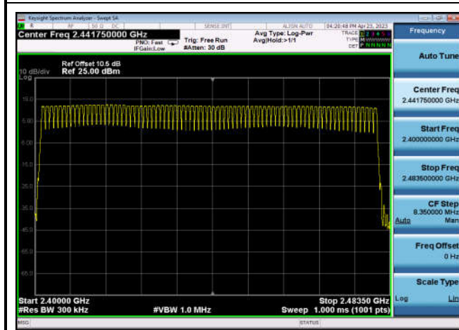
Number Of Hopping Channels: 8DPSK ,HoppingMhz,3DH5__2400~2483.5
