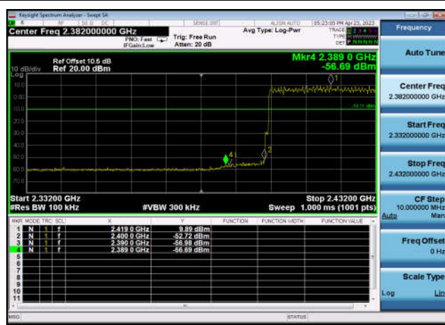
Conducted Emission: 8DPSK,2402,3DH5 ,Band Edge
