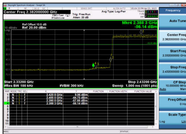
Conducted Emission: 8DPSK,2402,3DH5 ,Band Edge
