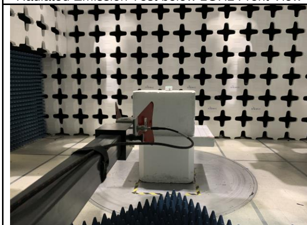
Radiated Emission Test Above 1GHz Front View
