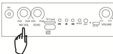
1. Turn the Mic Volume knob right to increase the sound and left to decrease the sound of the microphone.
