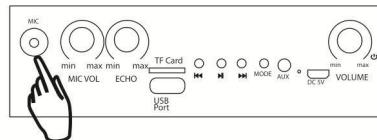
Plug in the included microphone's cable into the Mic Jack on the top of your speaker
