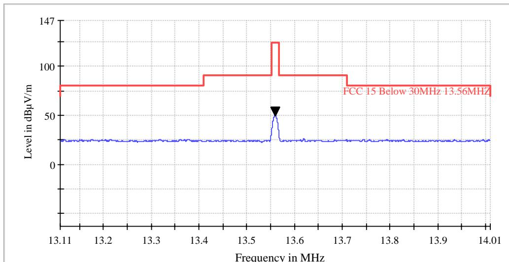
Radiated emission from 13.11MHz to 14.01MHz:
