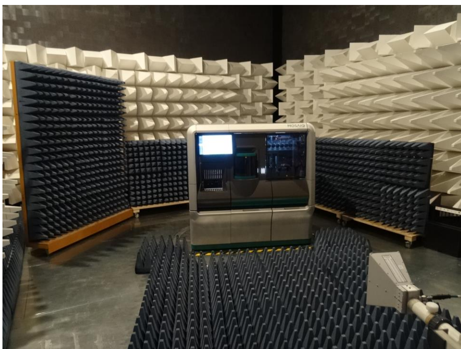
Figure 4 EUT / set up - test module ER2 (radiated emissions 1 - 18 GHz)
