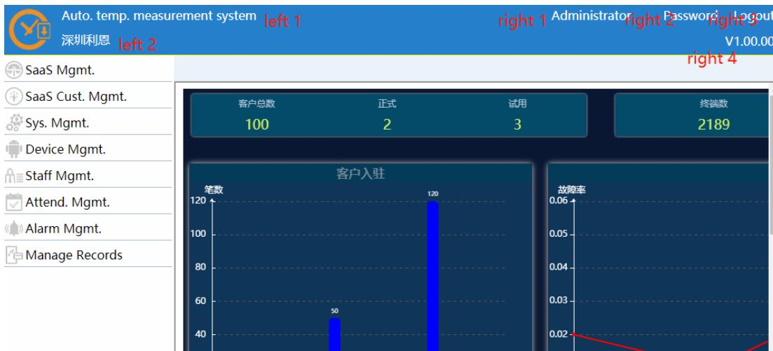
The main interface consists of three parts: comprehensive information area on the top, menu bar area on the left, and the main operation area on the right.
