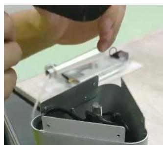
2. Remove the waterproof washer, corrugated elastic pad and nut from the *temperature measuring all-in-one machine* host and insert them into the top cover of sheet metal bracket. Then restore the waterproof washer, corrugated elastic pad and nut in order and tighten the nut.
