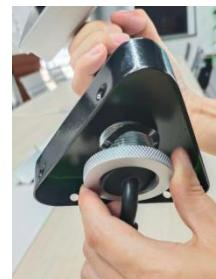
3. Connect the USB cable, network cable and DC power cord, and fasten the connector with electrical tape to prevent it from falling off.
