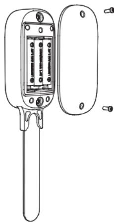
2. Insert the batteries and tighten the screw.
