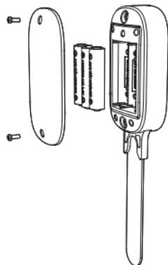
1. Unscrew the battery compartment.
