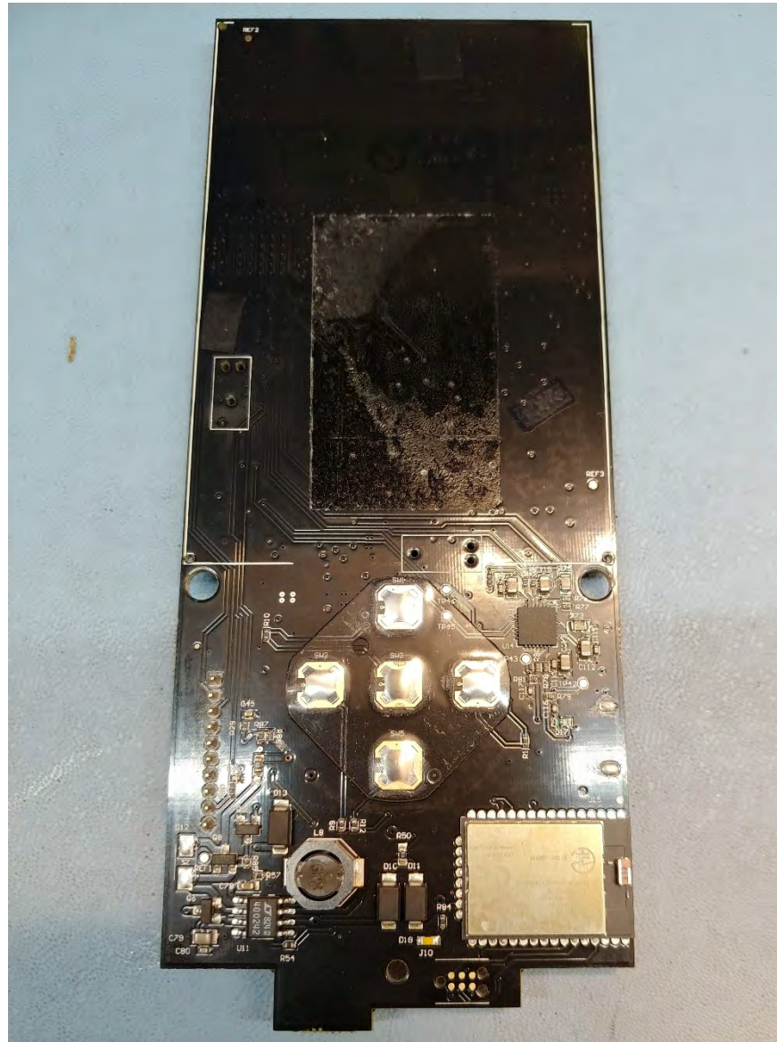
Front View – Mainboard with LCD removed
