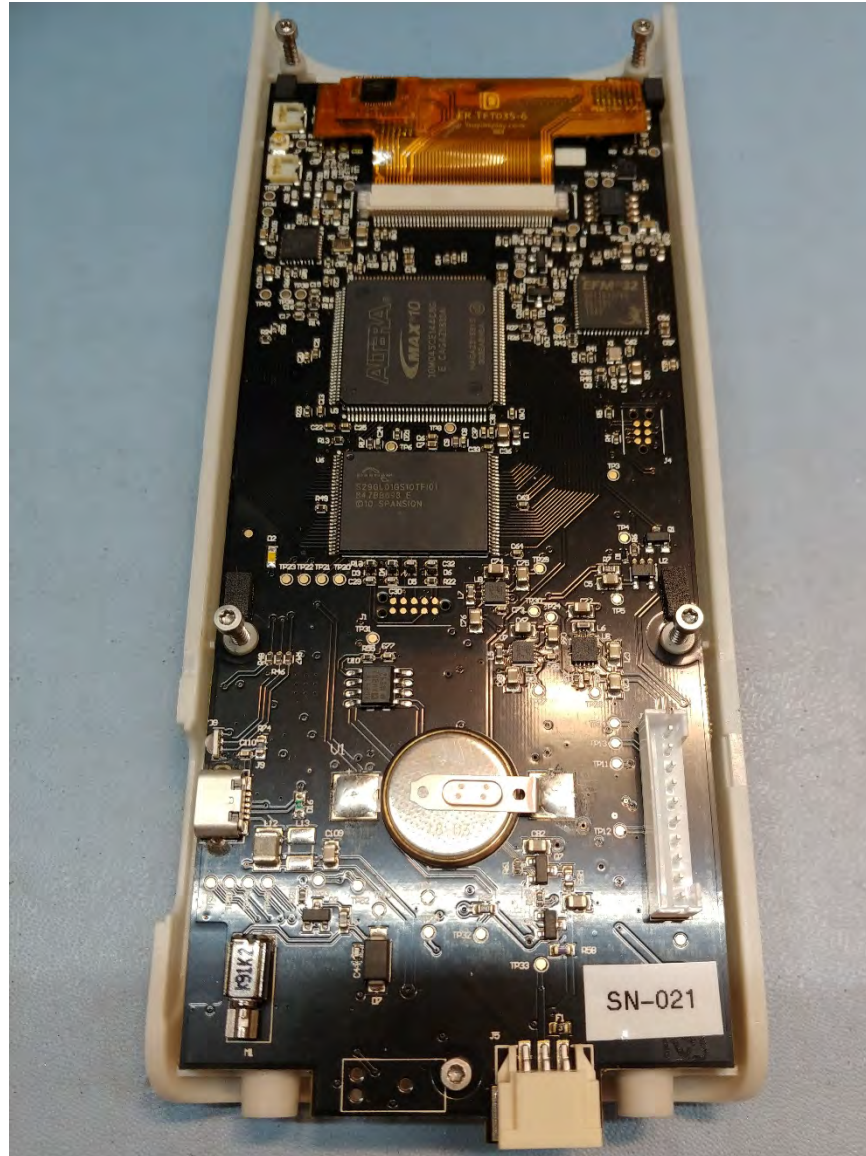
Rear View – Mainboard attached to Front Cover
