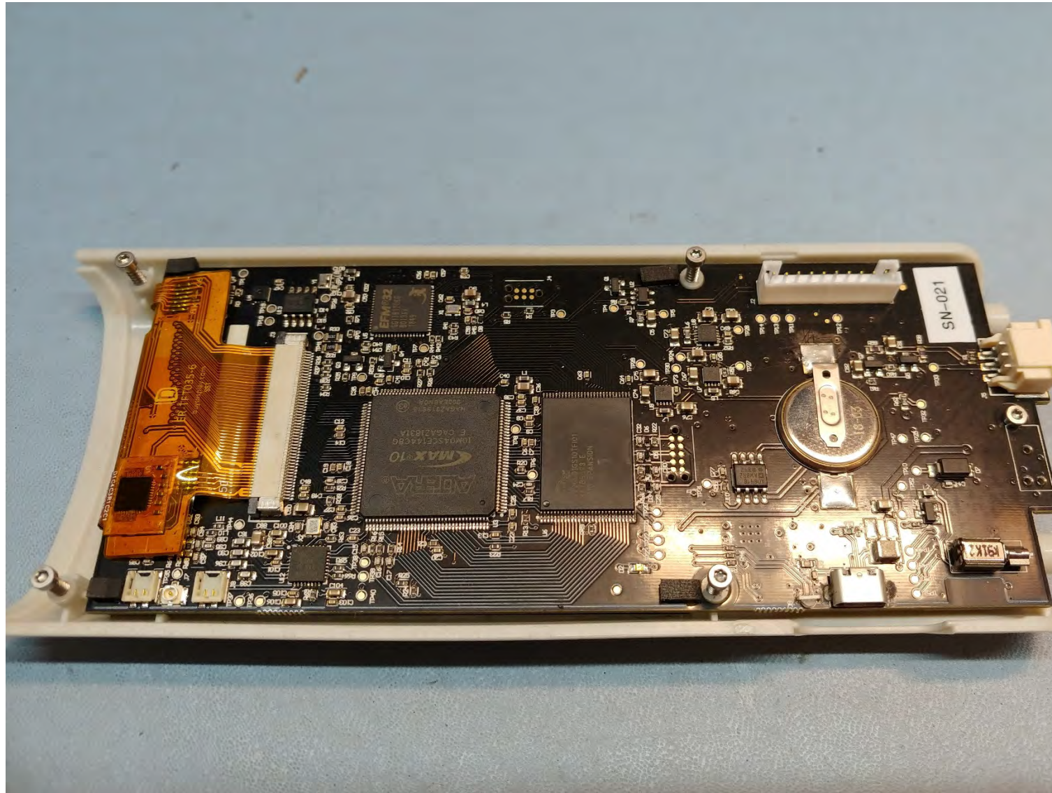
Right Side – Mainboard attached to Front Cover
