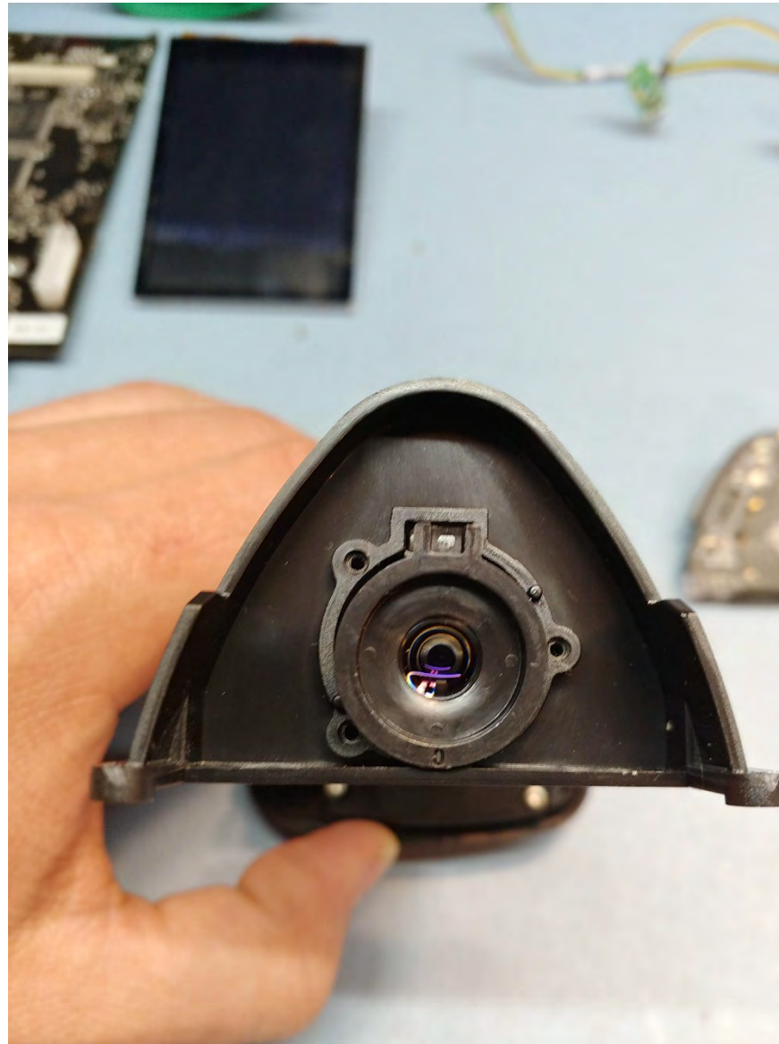
Bottom View – Optical Tube Lensing shown with Optical Board removed
