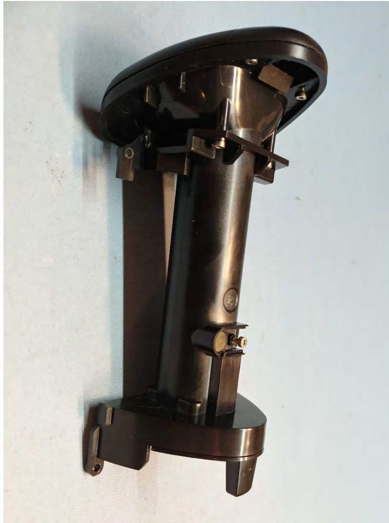
Right Side – Optical tube with Sampler Funnel attached
