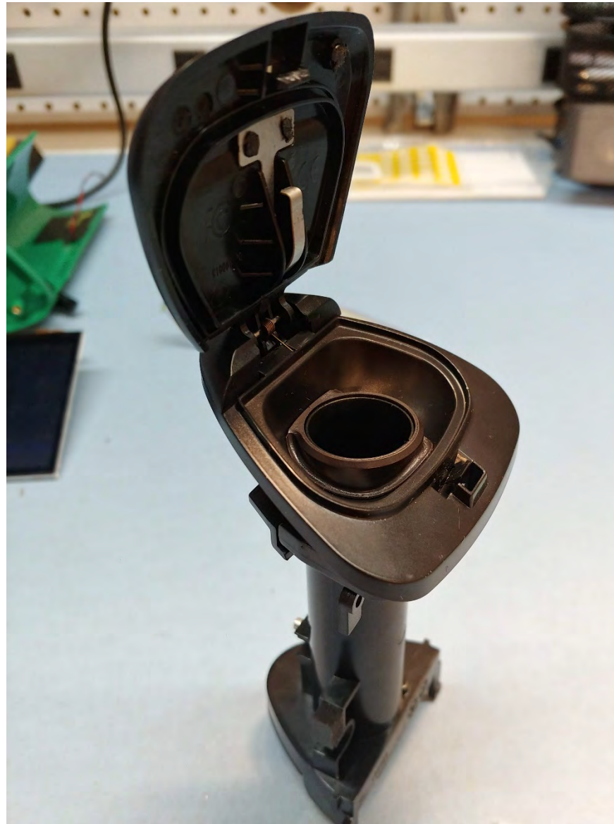
Left Side – Optical Tube and Sampler Funnel with Lid open
