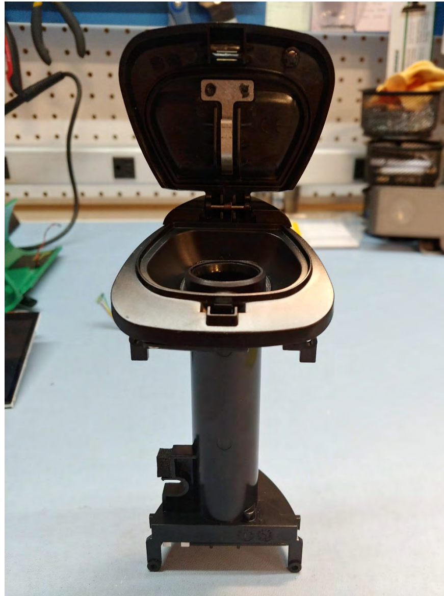
Front View– Optical Tube and Sampler Funnel with Lid open
