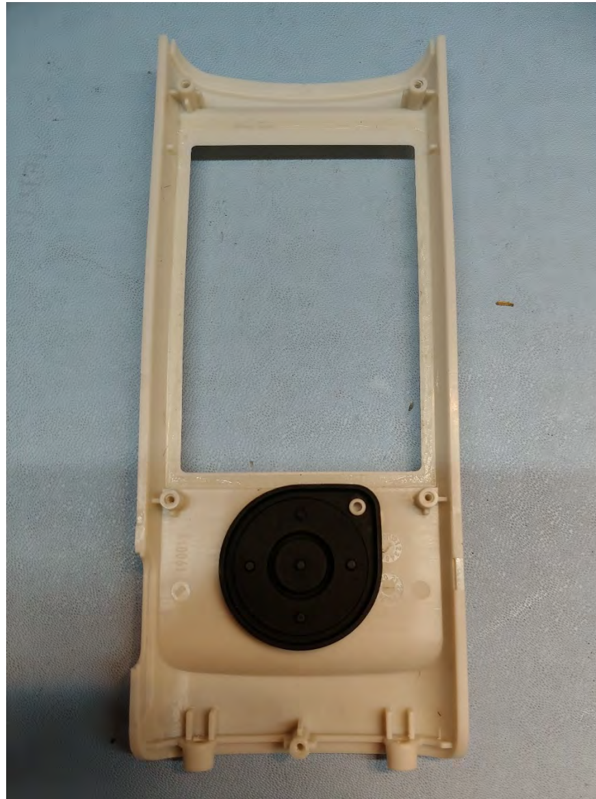
Rear View – Interior of Front Cover with Mainboard and LCD removed – Silicone Control Pad shown in black
