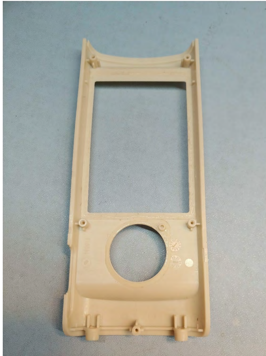
Rear View – Interior of Front Cover with Mainboard and LCD removed – Silicone Control Pad removed
