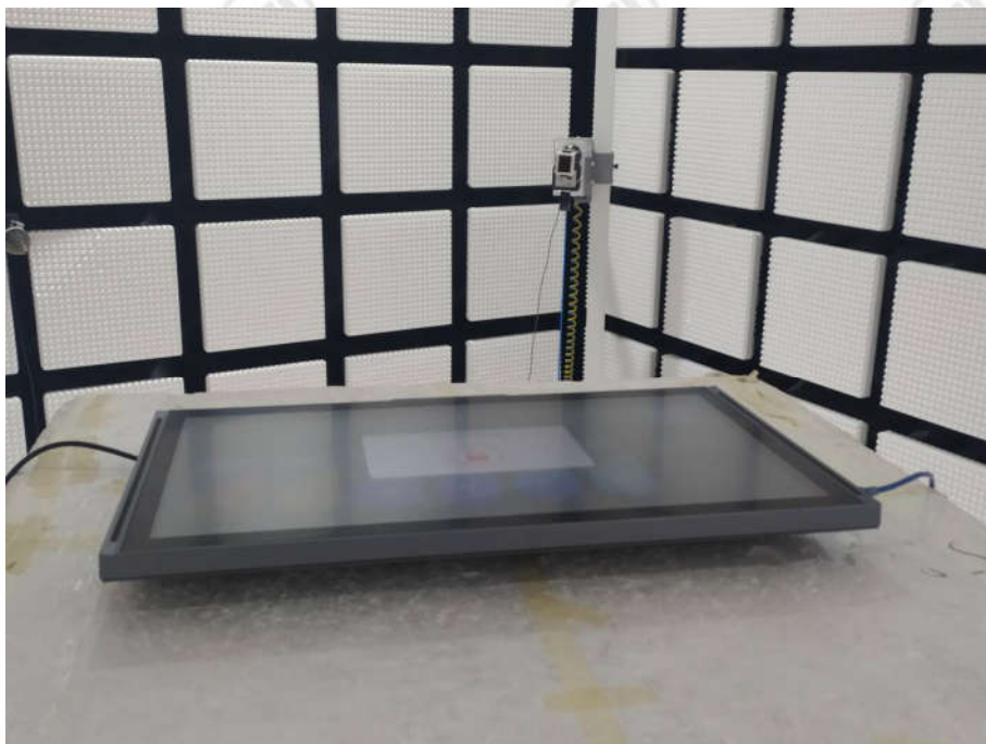
Radiated spurious emission Test Setup-3(Above 18GHz)
