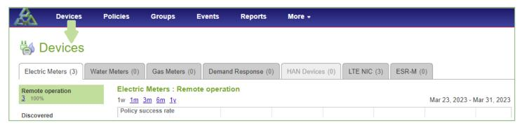
Devices include all the types of hardware, such as meters, communication cards, routers, and various edge devices, required to make the smart grid operational. The device types appear in tabs across the top of the Devices page.
