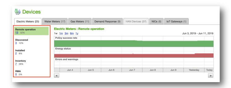
Operational states characterize stages in a device's life cycle, such as when it is in test mode, RMA, sitting in inventory, fielded but not in use, or fully fielded and in use. The operational states can also be used to dictate whether subscription billing is active for the device. The PolicyNet system uses the operational state to determine:
