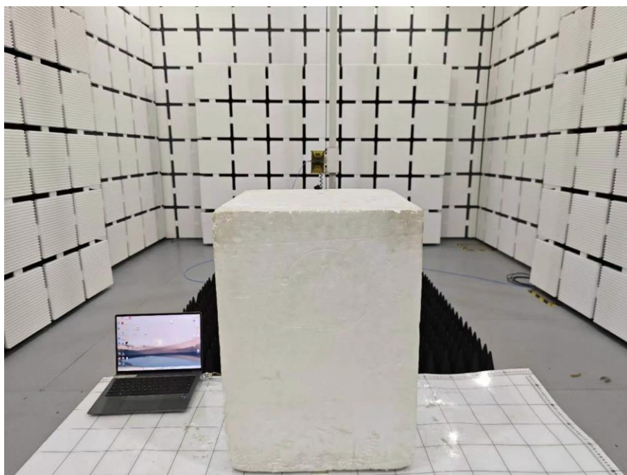
Set-up for Radiated Spurious Emission, Above 1GHz
