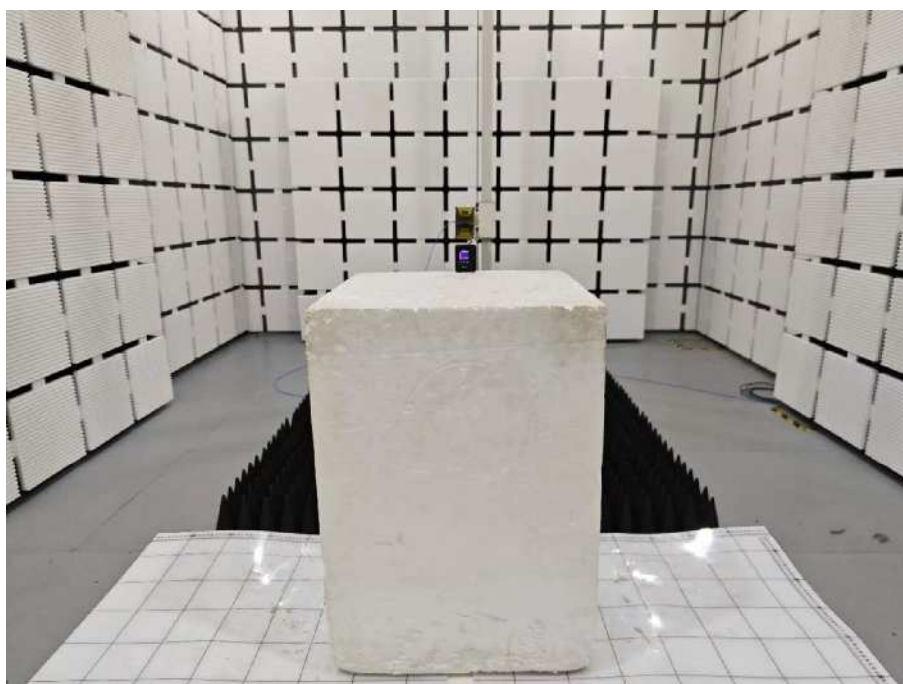
Set-up for Radiated Spurious Emission, Above 1GHz
