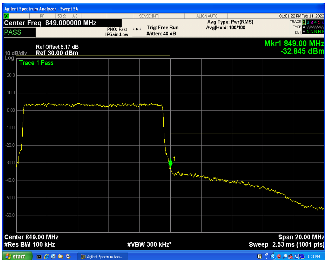
Band5 QAM16 BW=10MHz Channel=20600 RB Size=1 Position=#0
