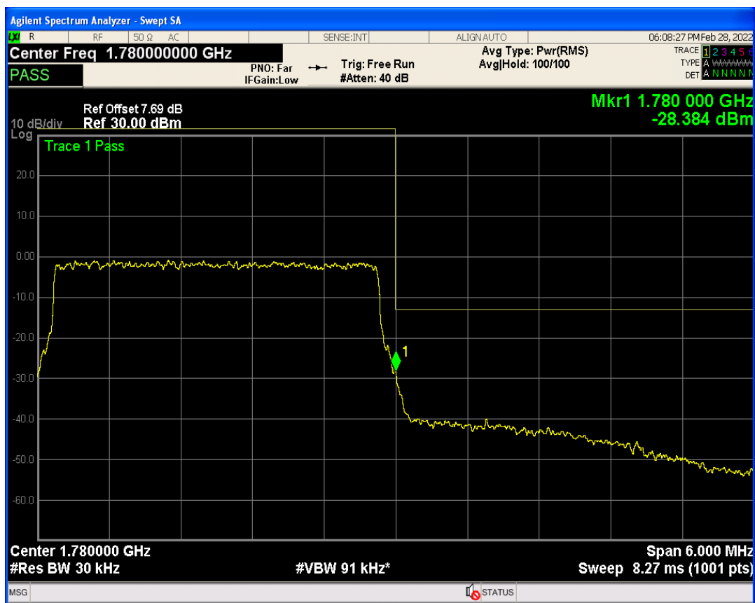
Band66 QAM16 BW=5MHz Channel=131997 RB Size=1 Position=#0
