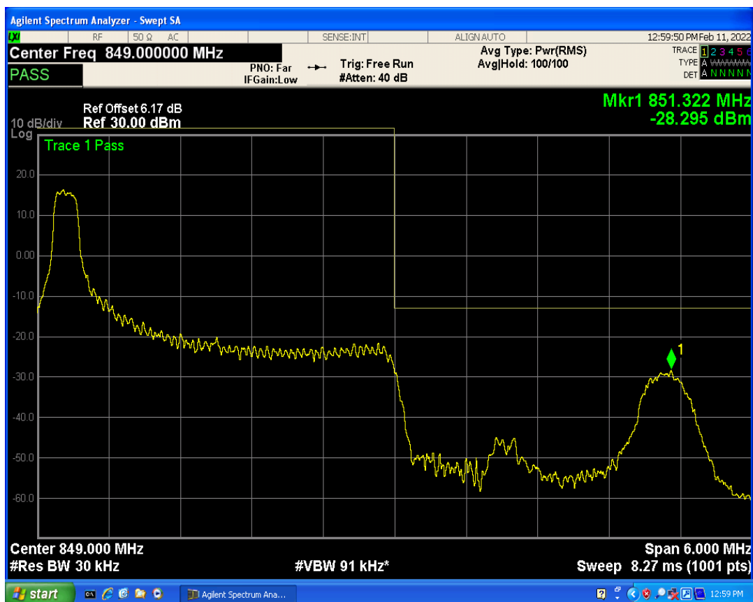
Band5 QAM16 BW=3MHz Channel=20635 RB Size=1 Position=#Max
