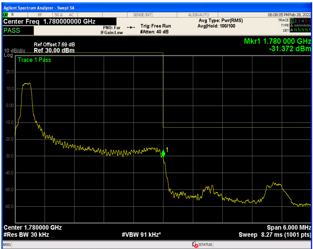
Band66 QPSK BW=5MHz Channel=131997 RB Size=1 Position=#0
