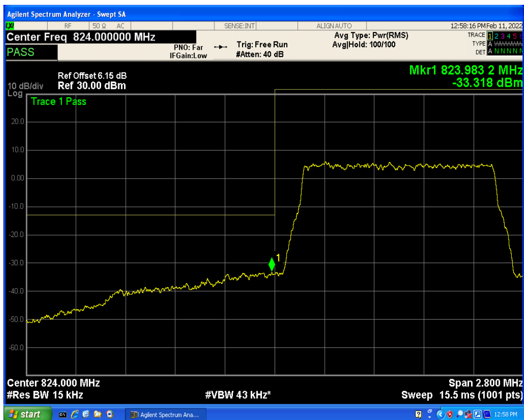
Band5 QAM16 BW=1.4MHz Channel=20407 RB Size=1 Position=#0
