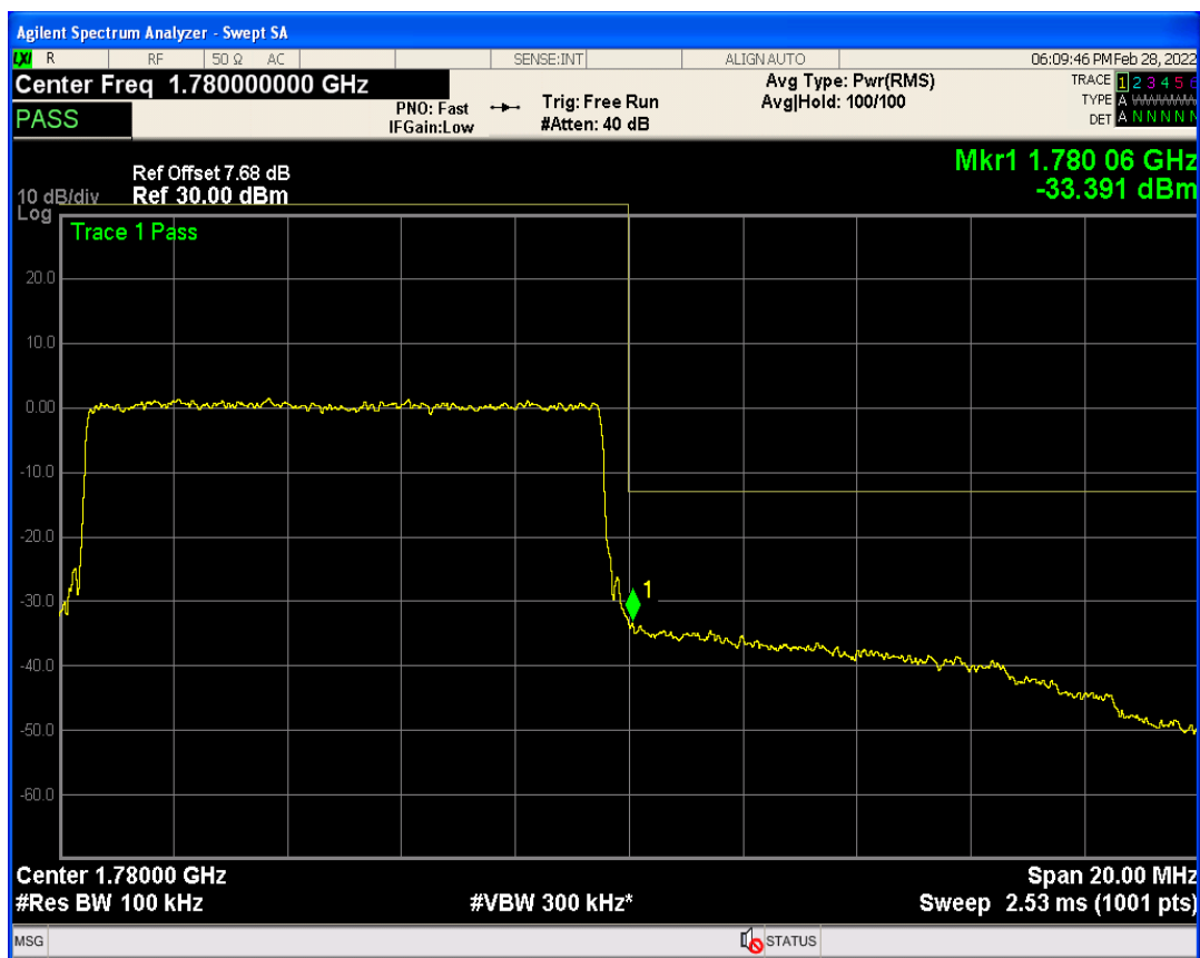
Band66 QPSK BW=15MHz Channel=132597 RB Size=1 Position=#Max
