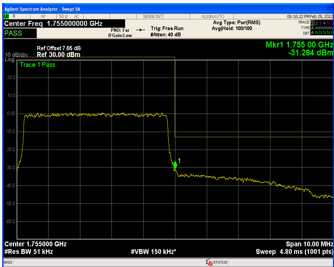
Band4 QPSK BW=5MHz Channel=20375 RB Size=1 Position=#Max
