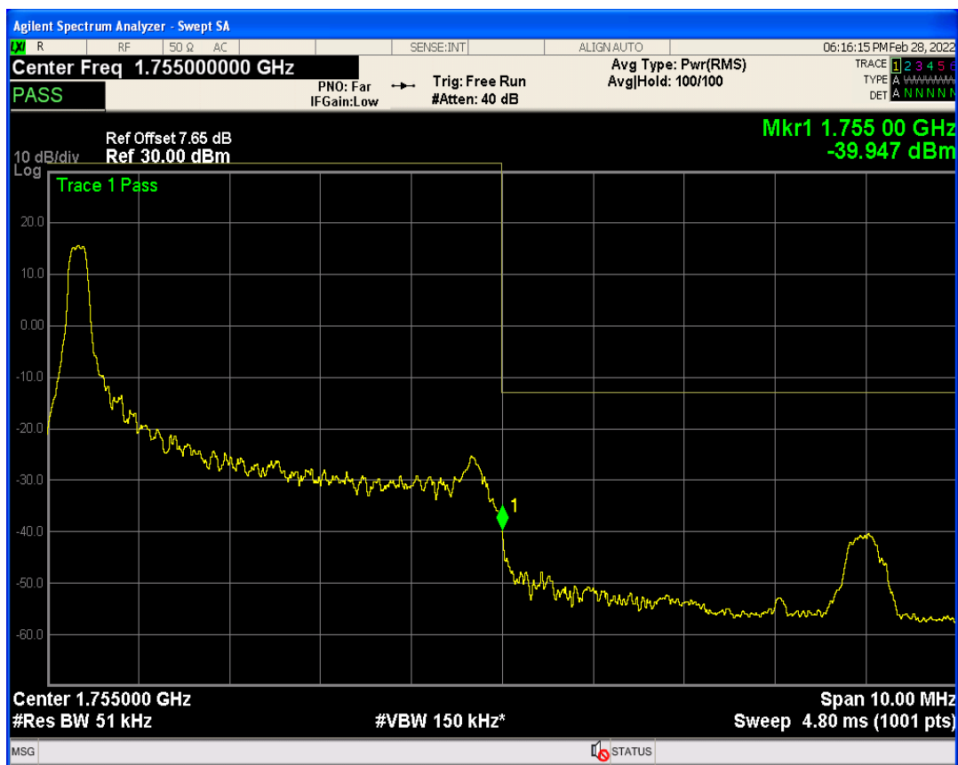
Band4 QPSK BW=3MHz Channel=19965 RB Size=1 Position=#0
