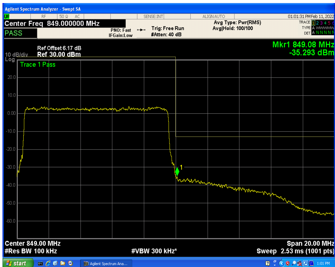
Band66 QAM16 BW=1.4MHz Channel=132665 RB Size=6 Position=#0
