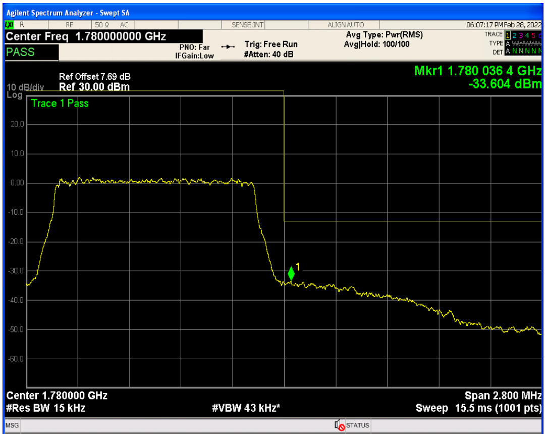
Band66 QPSK BW=1.4MHz Channel=131979 RB Size=6 Position=#0
