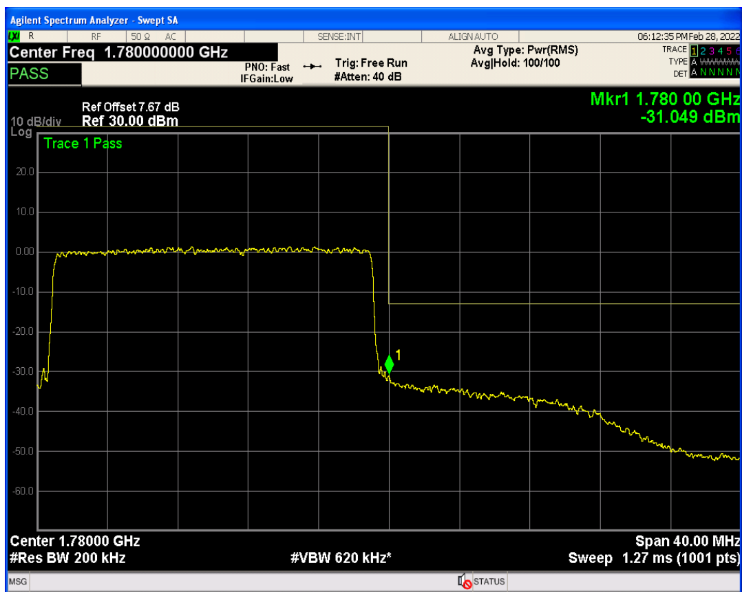
Band66 QPSK BW=3MHz Channel=131987 RB Size=1 Position=#0
