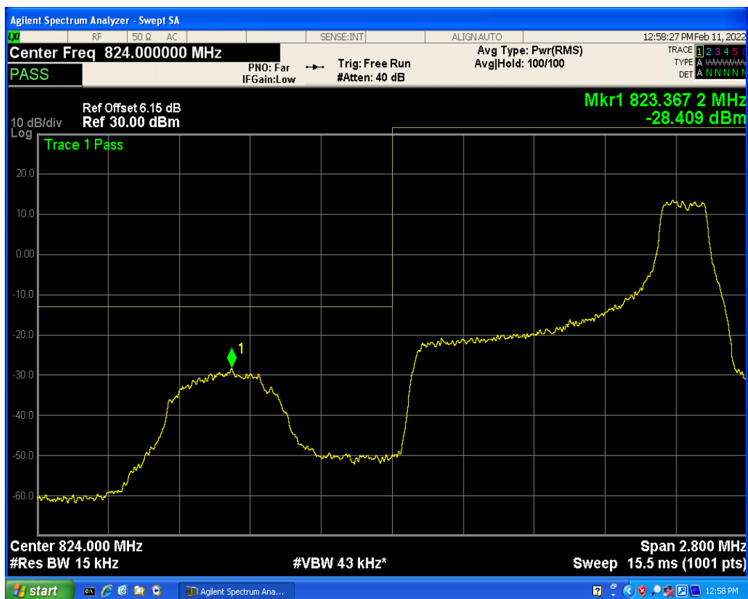
Band5 QPSK BW=1.4MHz Channel=20643 RB Size=1 Position=#0
