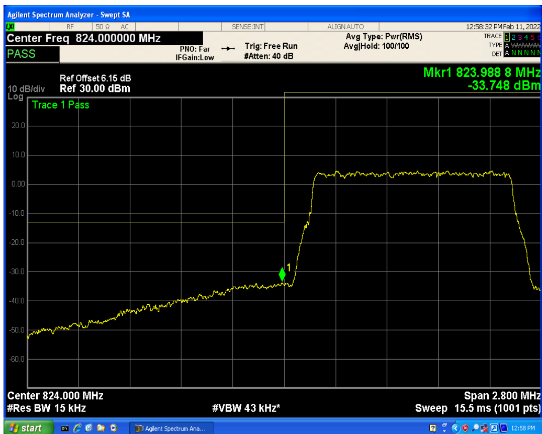
Band5 QPSK BW=1.4MHz Channel=20643 RB Size=1 Position=#Max
