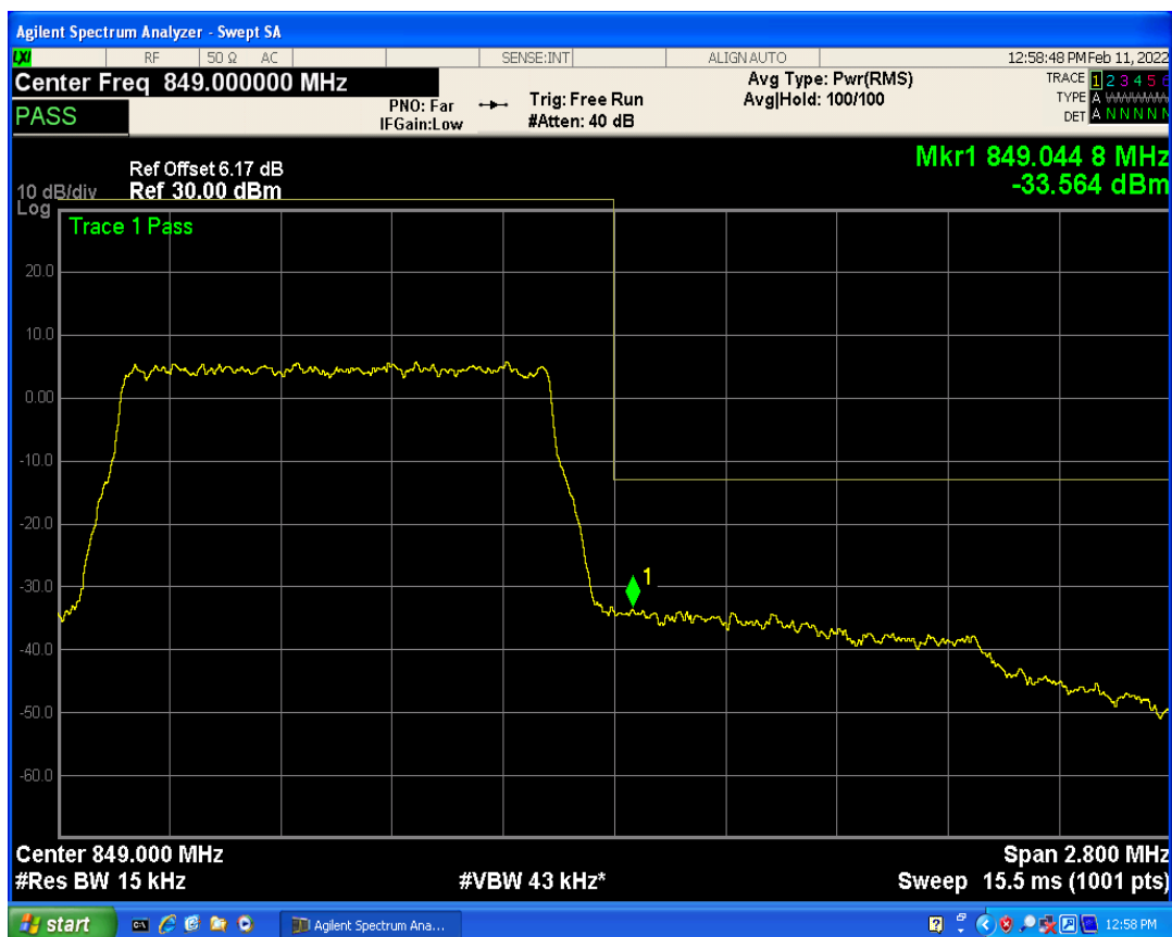
Band5 QAM16 BW=1.4MHz Channel=20643 RB Size=1 Position=#Max
