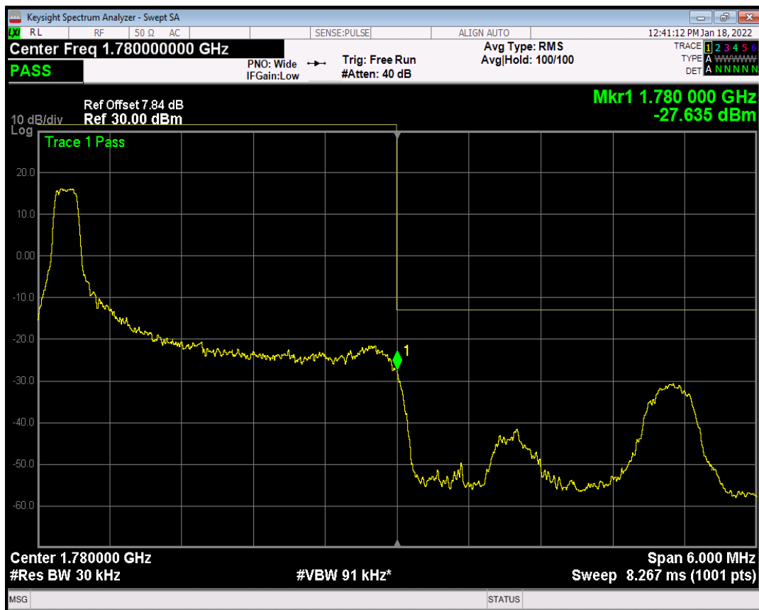
Band66 QAM16 BW=3MHz Channel=131987 RB Size=15 Position=#0
