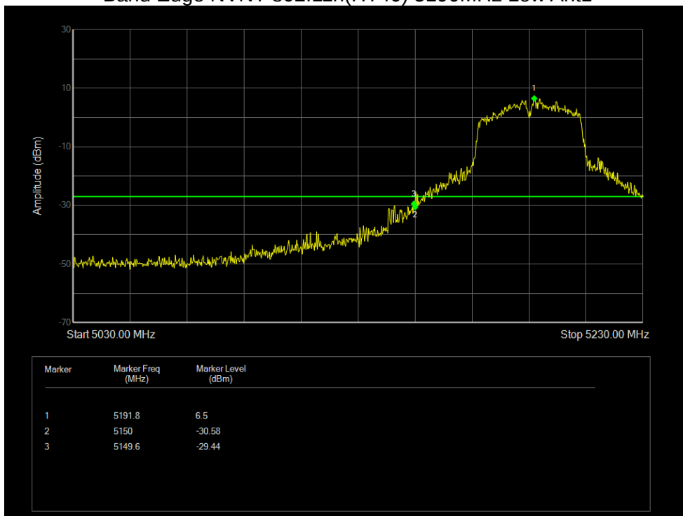
Band Edge NVNT 802.11n(HT40) 5190MHz Low Ant1
