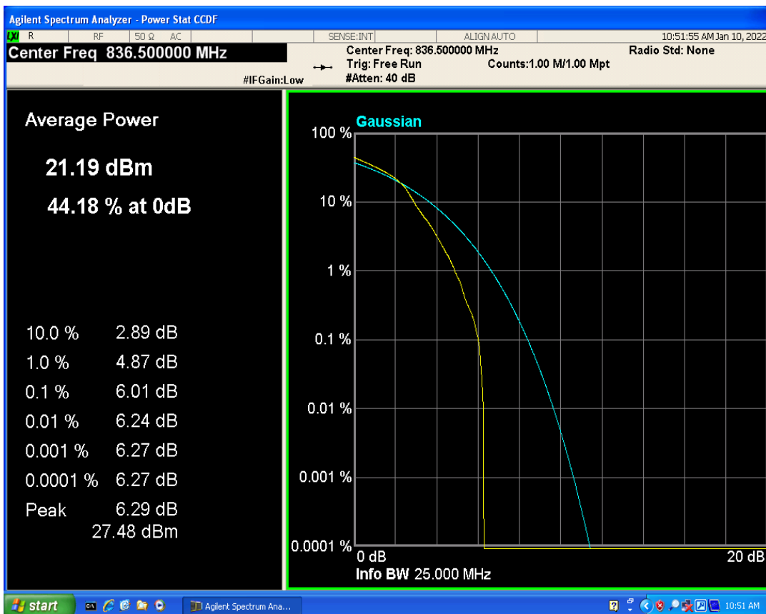
Band5 QPSK BW=3MHz Channel=20525 RB Size=1 Position=#0
