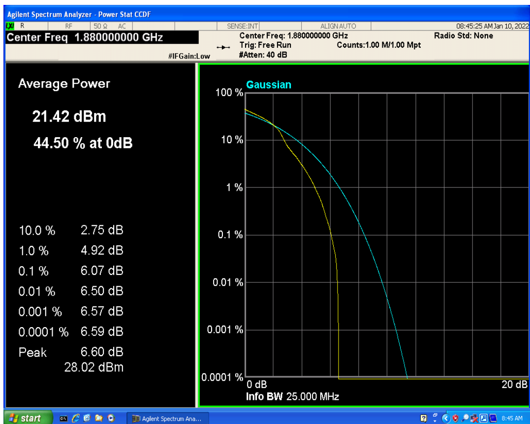
Band2 QPSK BW=15MHz Channel=18900 RB Size=1 Position=#0
