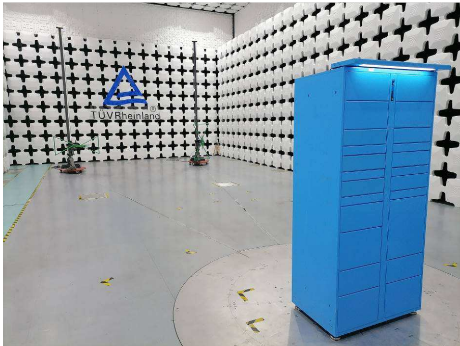
Photograph 1: Set-up photo for Radiated Emission, Below 1GHz
