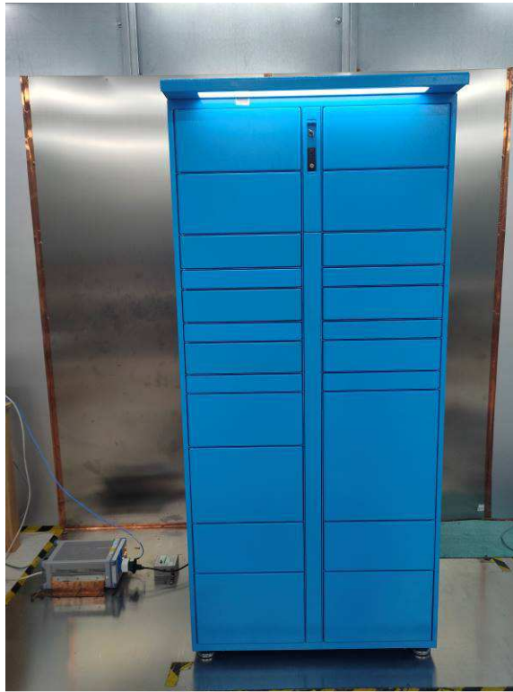
Photograph 3: Set-up photo for Conducted Emissions on AC Mains
