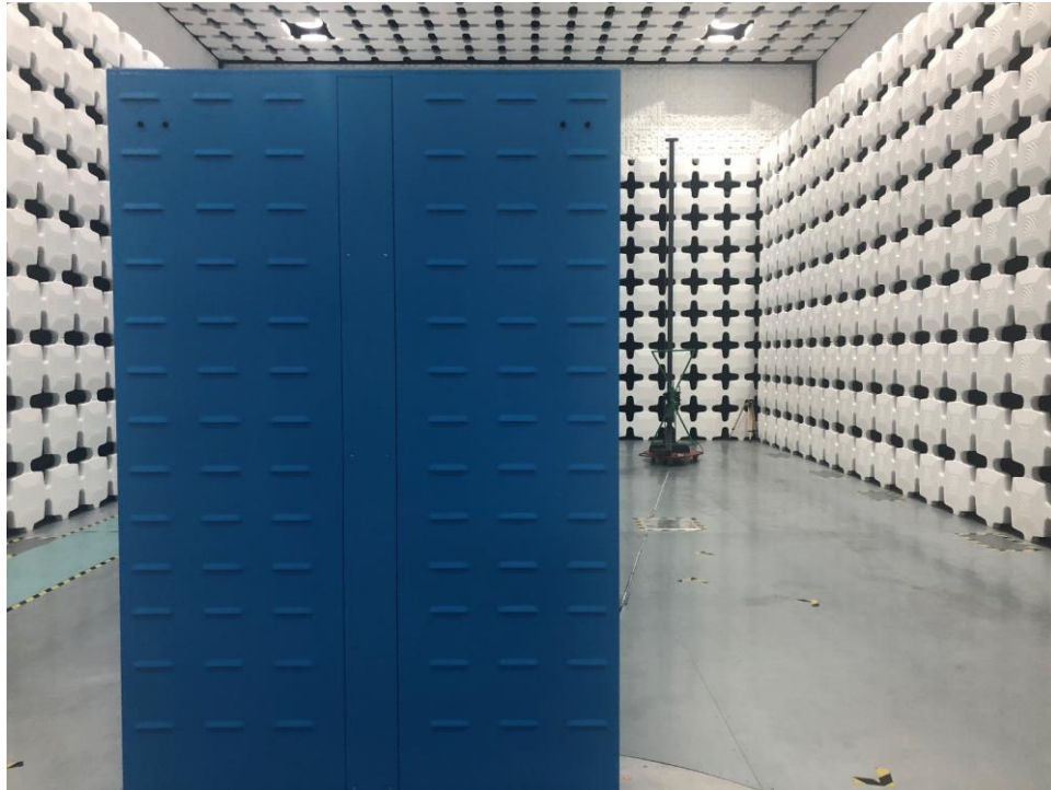
Photograph 1: Set-up for Radiated Emission, Below 1GHz
