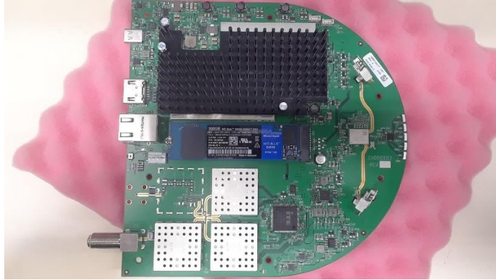
Top of Internal board including Antenna positions
