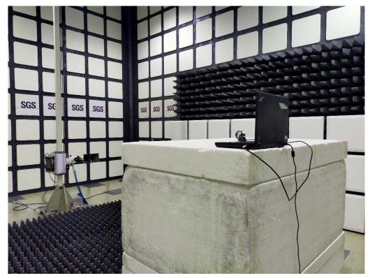
Radiated Emission Set up Photos (Front View)
